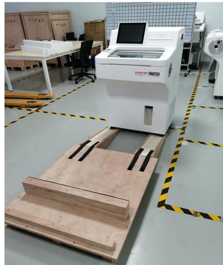
Figure d Move the instrument to the floor
