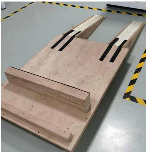
Figure c Dismantle the crate, remove the EPE, and set up a slope
