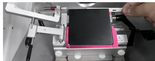
2) Unfold the anti-roll guide
